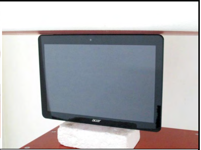
Top Side of EUT with 0 cm Gap
