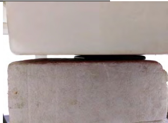
Fig.3 EUT Back side to flat phantom
