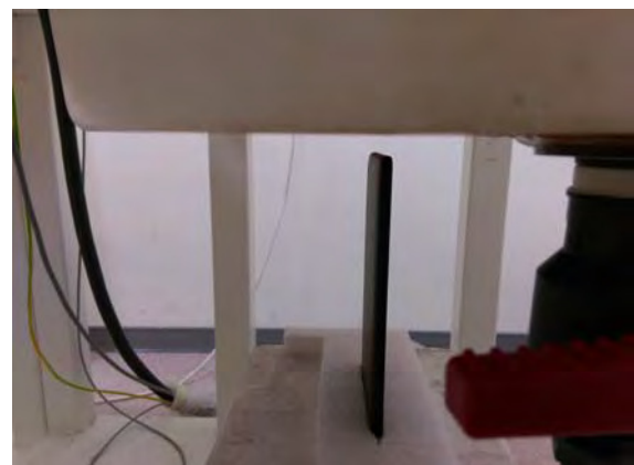
Fig.7 EUT Top side (13mm) to flat phantom
