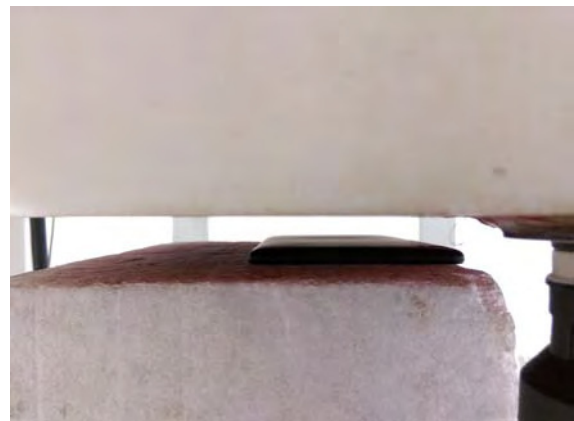
Fig.4 EUT Back side (17mm) to flat phantom
