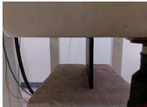
Fig.5 EUT Right side to flat phantom
