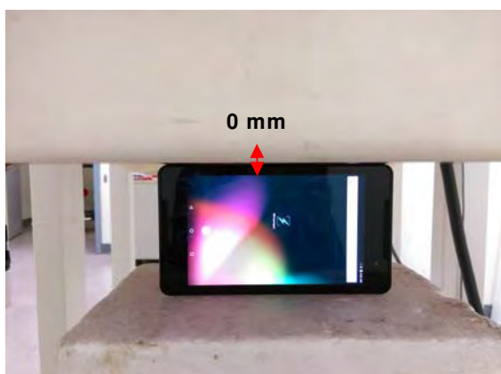
Fig.8 EUT Left side to flat phantom
