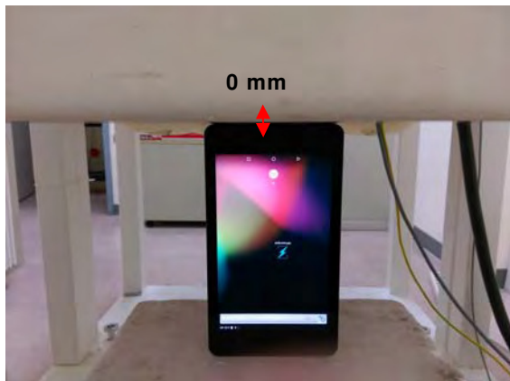
Fig.10 EUT Bottom side to flat phantom
