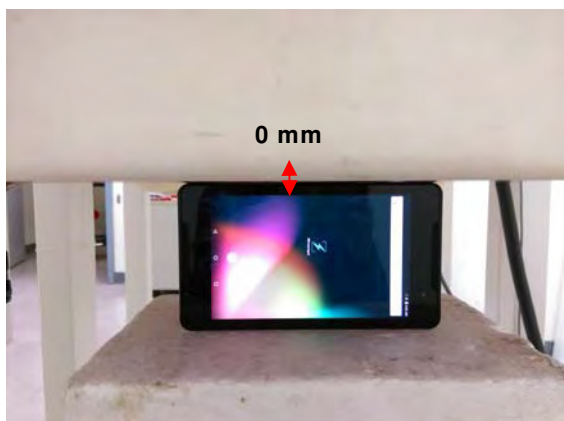
Fig.8 EUT Left side to flat phantom
