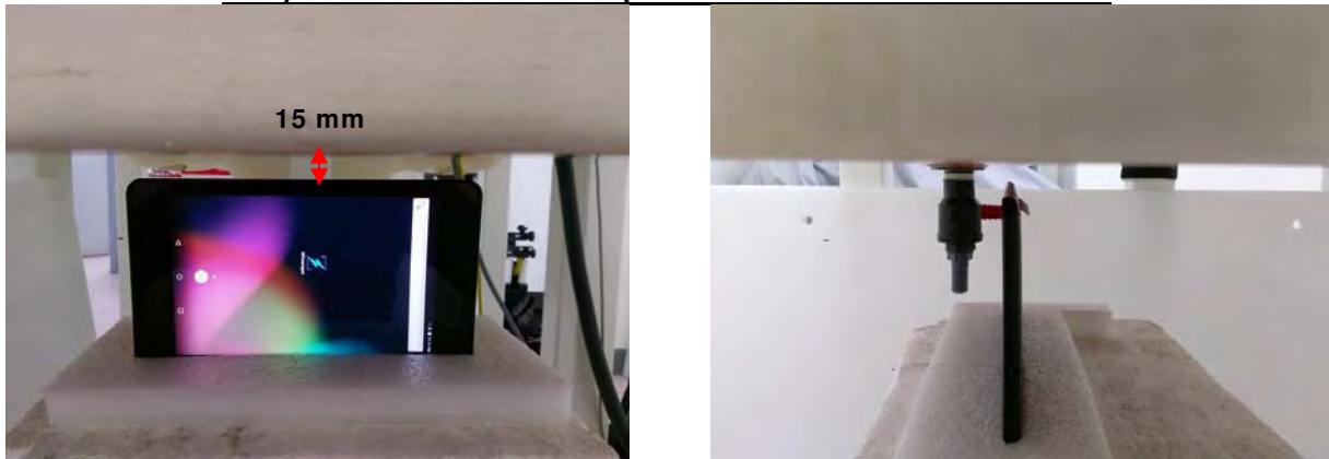
Fig.9 EUT Left side (15mm) to flat phantom
