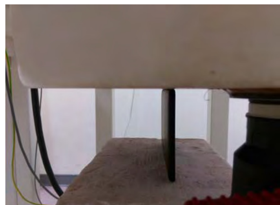
Fig.8 EUT Left side to flat phantom
