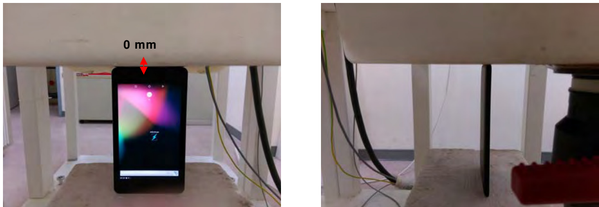
Fig.10 EUT Bottom side to flat phantom
