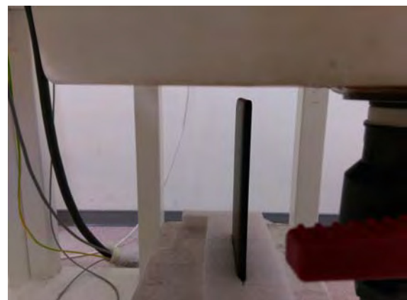
Fig.7 EUT Top side (13mm) to flat phantom
