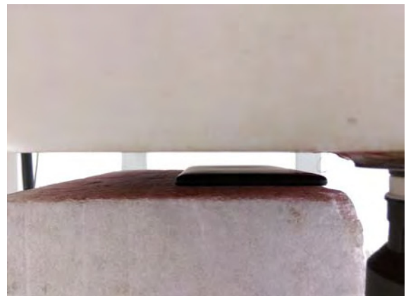
Fig.4 EUT Back side (17mm) to flat phantom
