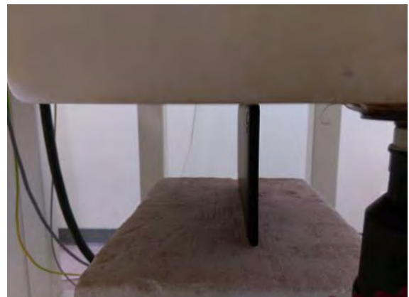
Fig.5 EUT Right side to flat phantom
