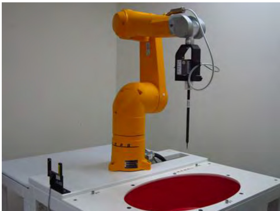
Fig.1 Photograph of the SAR measurement system
