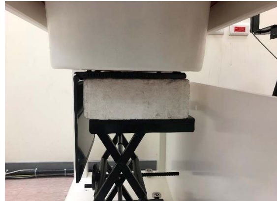
Fig.3 EUT Bottom side to flat phantom
