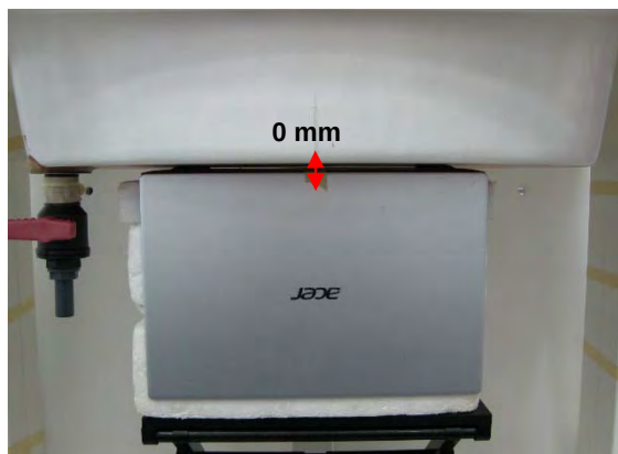
Fig.3 EUT Bottom side to flat phantom
