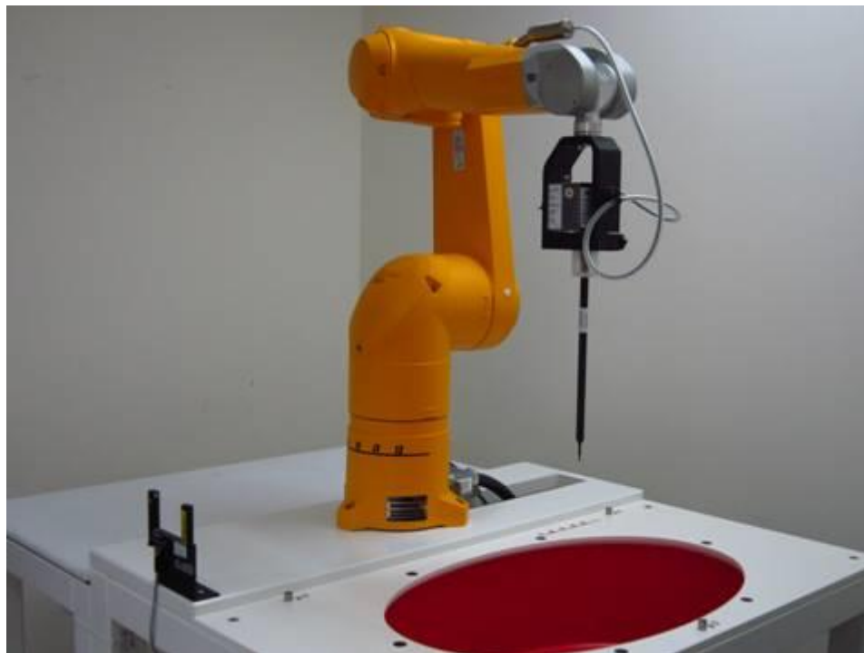
Fig.1 Photograph of the SAR measurement system
