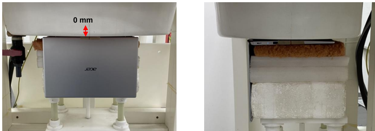
Fig.3 EUT Bottom side to flat phantom
