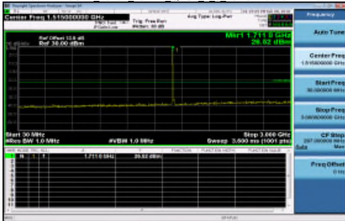
3GHz~10GHz Band4 15MHz QPSK 1 0 LowCH20025-1717.5
