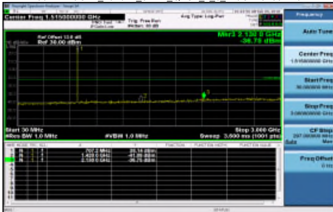
30MHz~3GHz Band17 5MHz QPSK 1_0 MidCH23790-710
