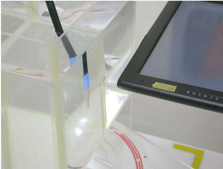
Figure: 12 EUT right to phantom, 15 mm separation
