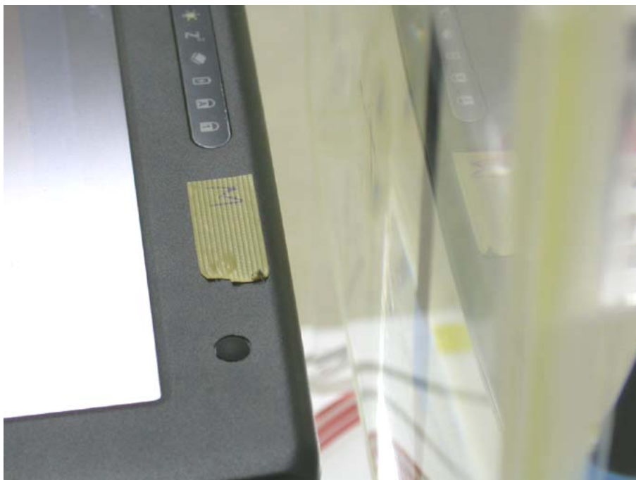
Figure: 5 EUT top to phantom, 15 mm separation – Zoom In
