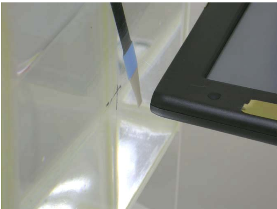
Figure: 13 EUT right to phantom, 15 mm separation– Zoom In
