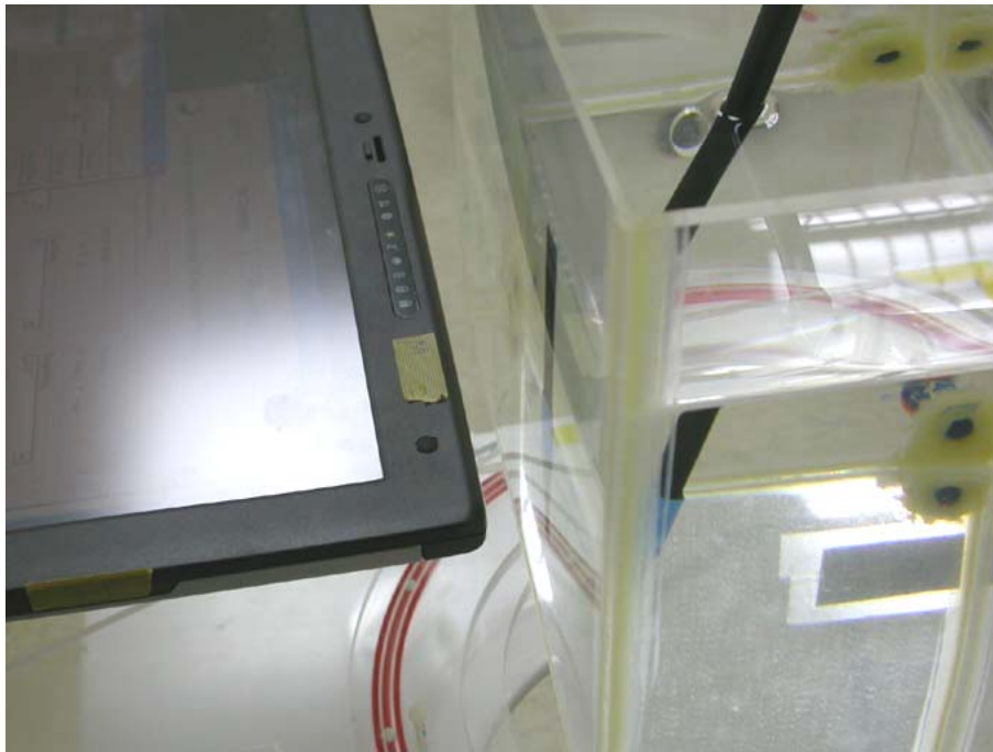
Figure: 4 EUT top to phantom, 15 mm separation
