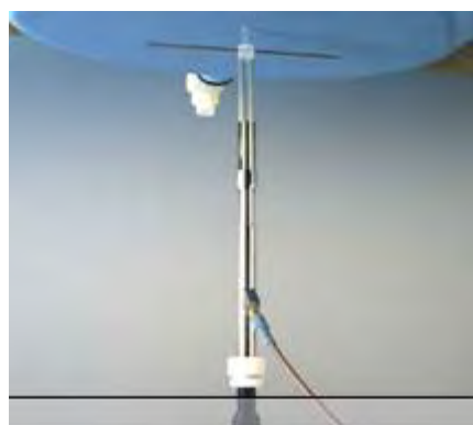
Photograph of the dipole Antenna
