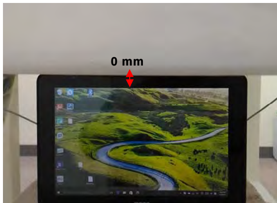
Fig.3 EUT Top side to flat phantom
