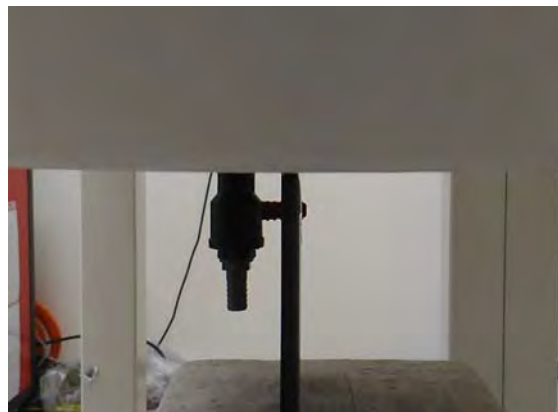
Fig.3 EUT Top side to flat phantom
