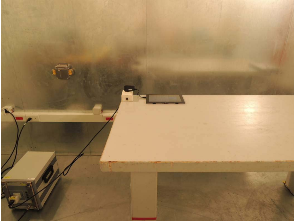
Conduction Setup Photo (Measurement at AC Power Line )-1
