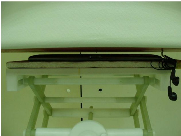
Bottom Face of Tablet with Phantom 0.5 cm Gap
