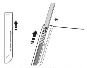
2 Push the switch to the left. The LED lights up when 3G is enabled.
