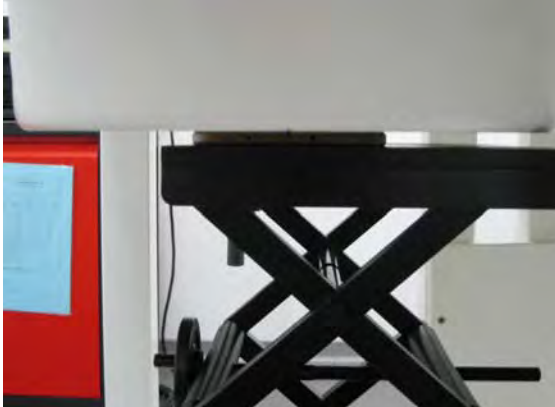
Fig.3 EUT Lap-held mode to flat phantom
