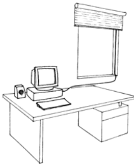
An example of start-up antenna placement
