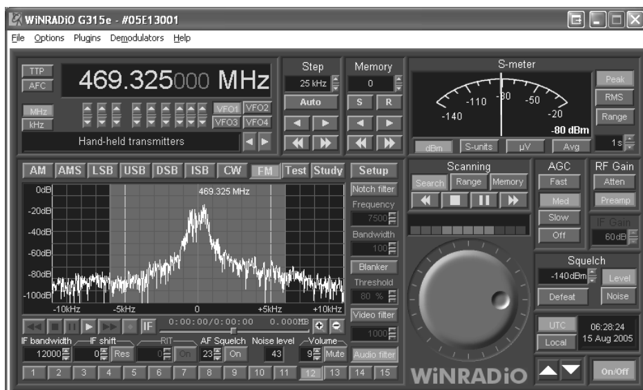
WiNRADiO G3XX Receiver Control Panel
