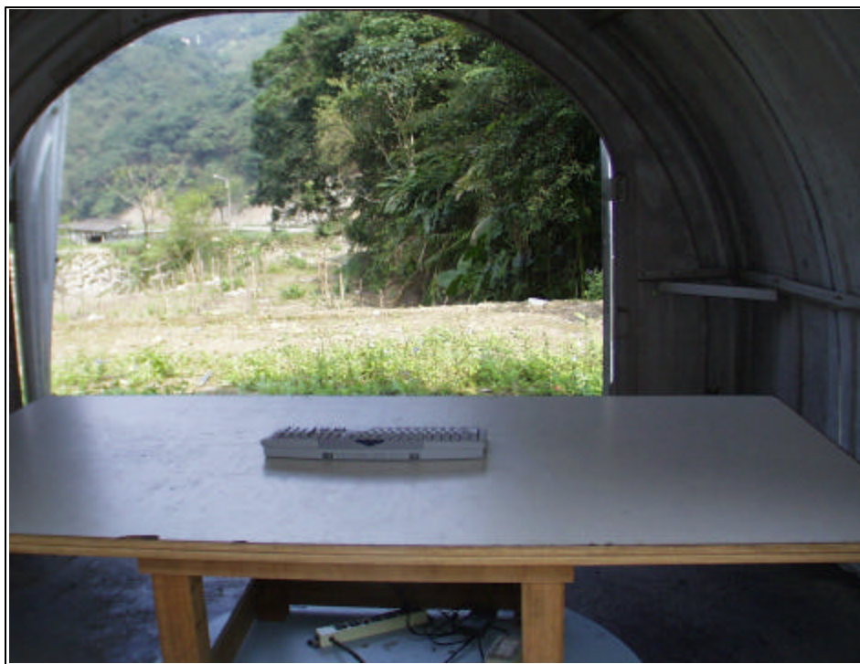
Radiated Open Site Test Set-up
