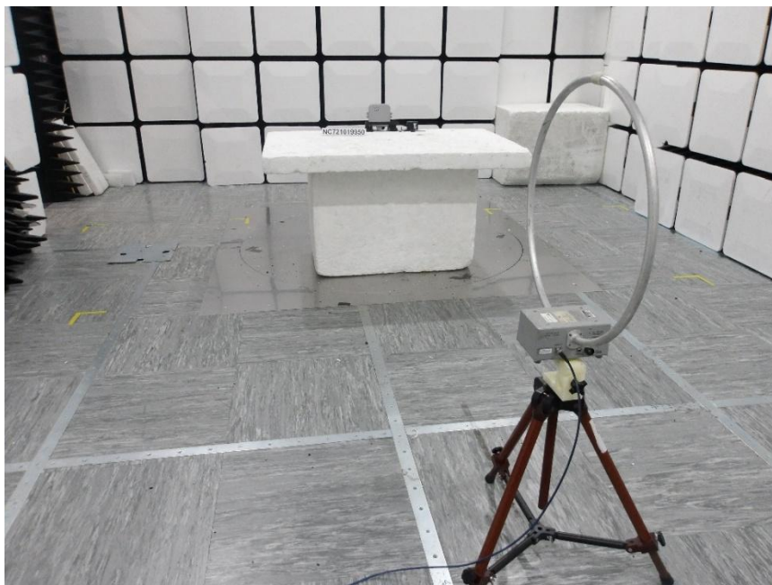
Photo 1-3 – Radiated Spurious Emissions 9 kHz-30 MHz – Front View [Vertical Co-Planar]
