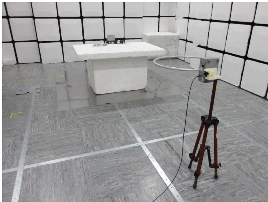
Photo 1-5 – Radiated Spurious Emissions 9 kHz-30 MHz – Front View [Horizontal Co-Planar]
