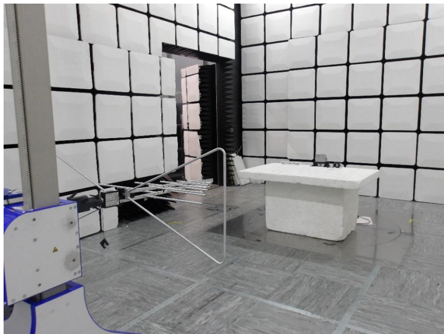
Photo 1-7 – Radiated Spurious Emissions 30MHz – 1GHz – Front View
