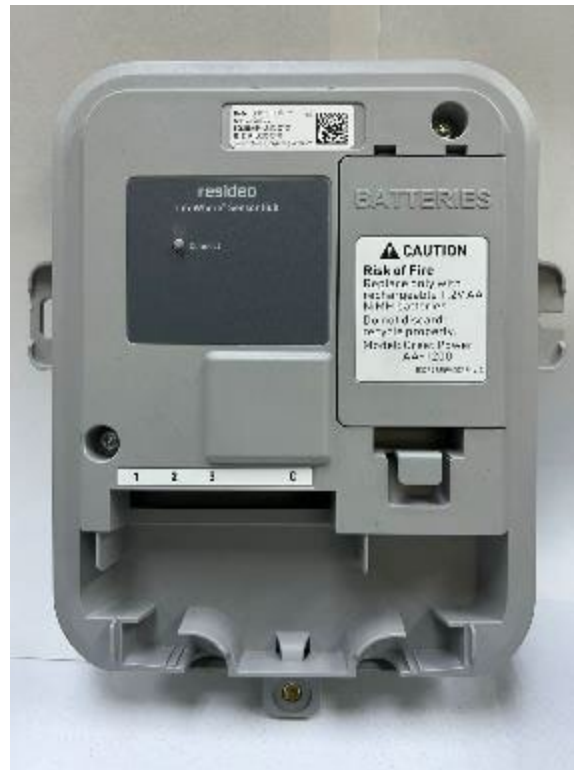
Figure 3 Assembly case back with battery compartment
