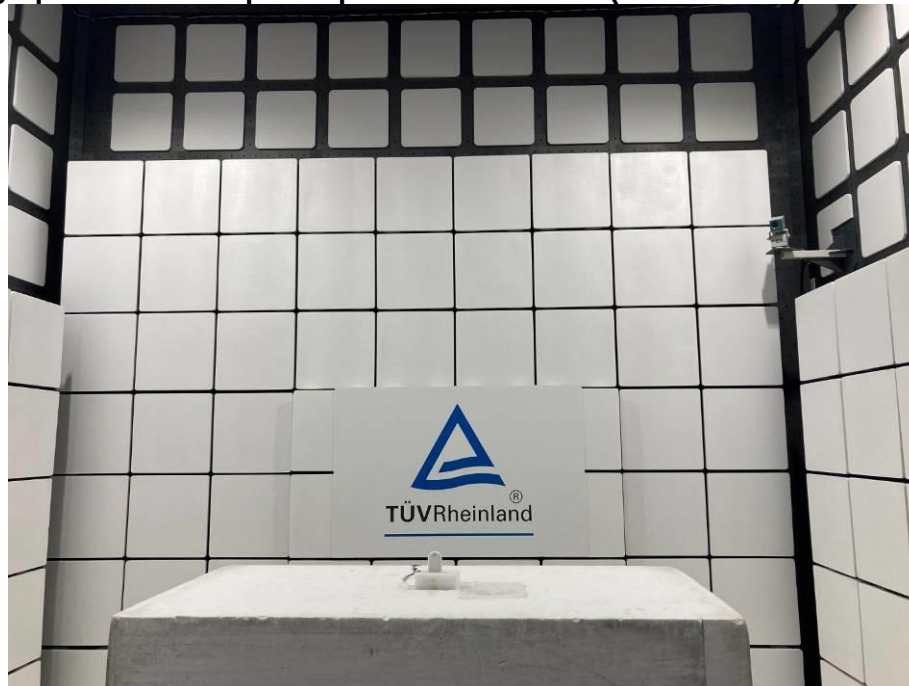
Photograph 2: Test Setup for Spurious Emissions (Front View 2)
