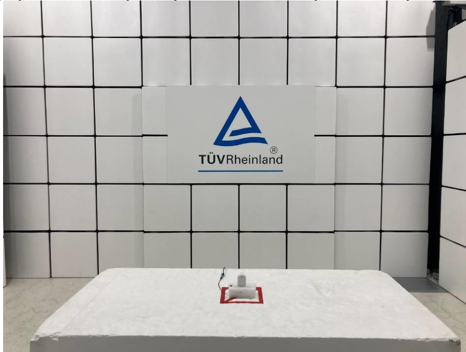
Photograph 2: Test Setup for Spurious Emissions (Front View 2)
