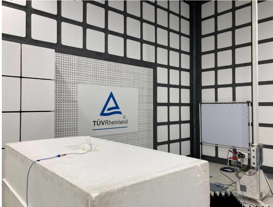
Photograph 6: Test Setup for Spurious Emissions (Back View 4)
