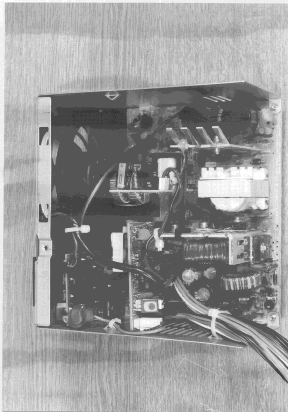
8.22 Power supply Minebea, opened case, inside view
