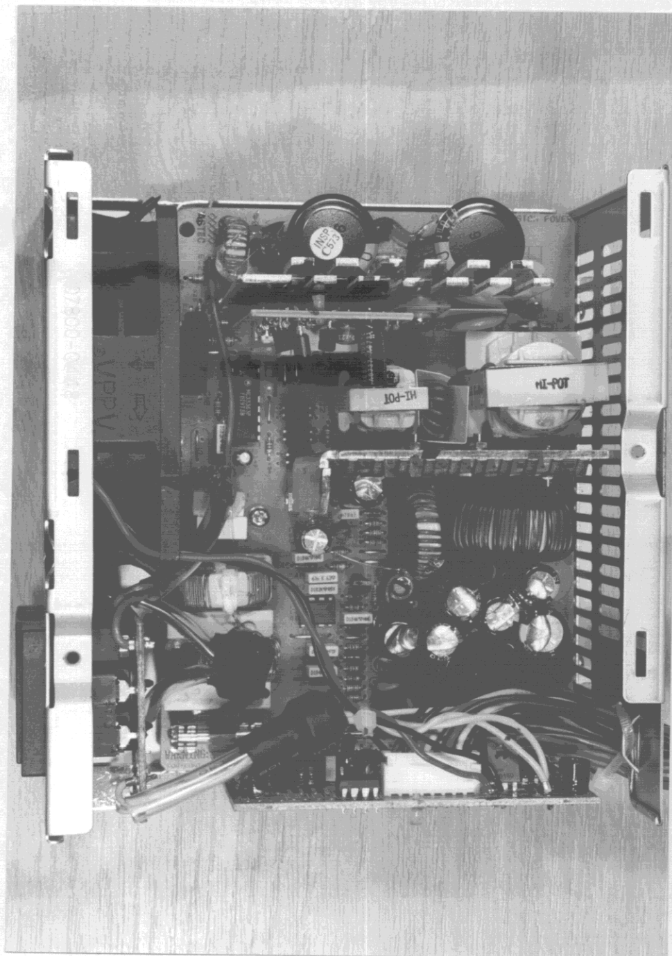
8.18 Power supply ASTEC, opened case, inside view
