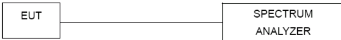
Figure 7. Conducted Bandedge Test Configuration
