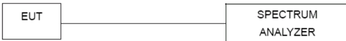
Figure 2. Conducted Radio Setup
