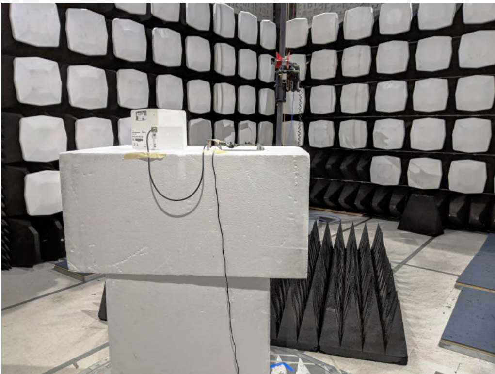
Figure 6: Equipment Under Test – Radiated Emissions – >1GHz
