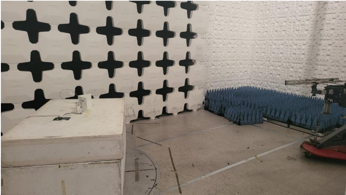
Figure 11. Radiated Emissions with Corner Reflector, 200-1000 MHz
