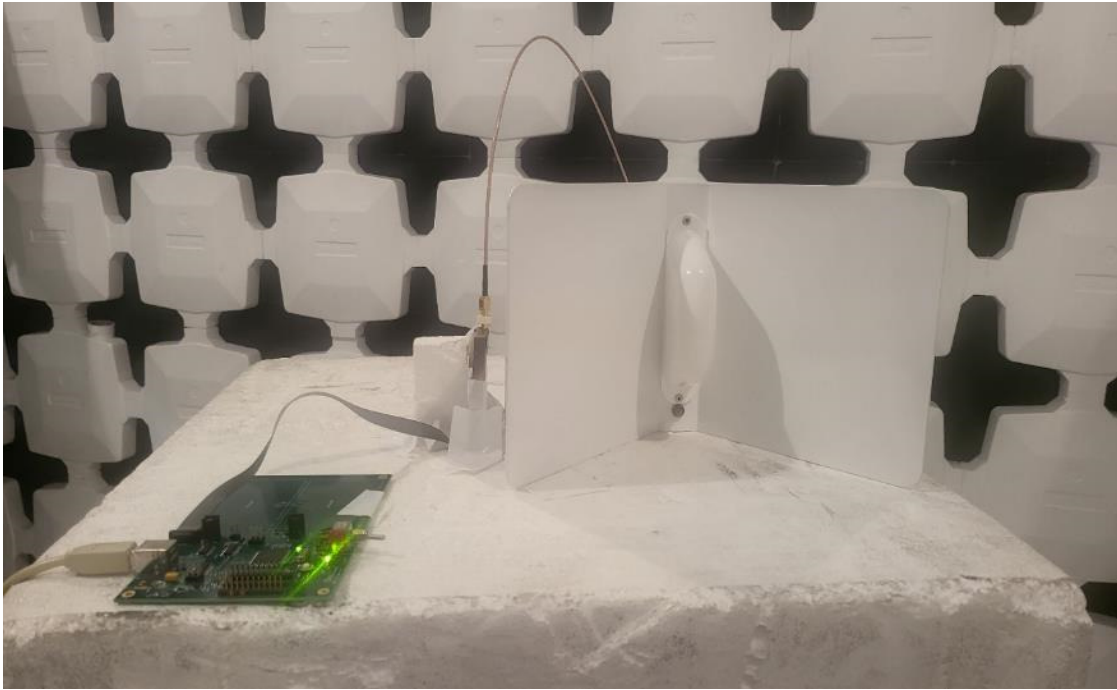
Figure 7. EUT Setup Fundamental Emissions, with Corner Reflector
