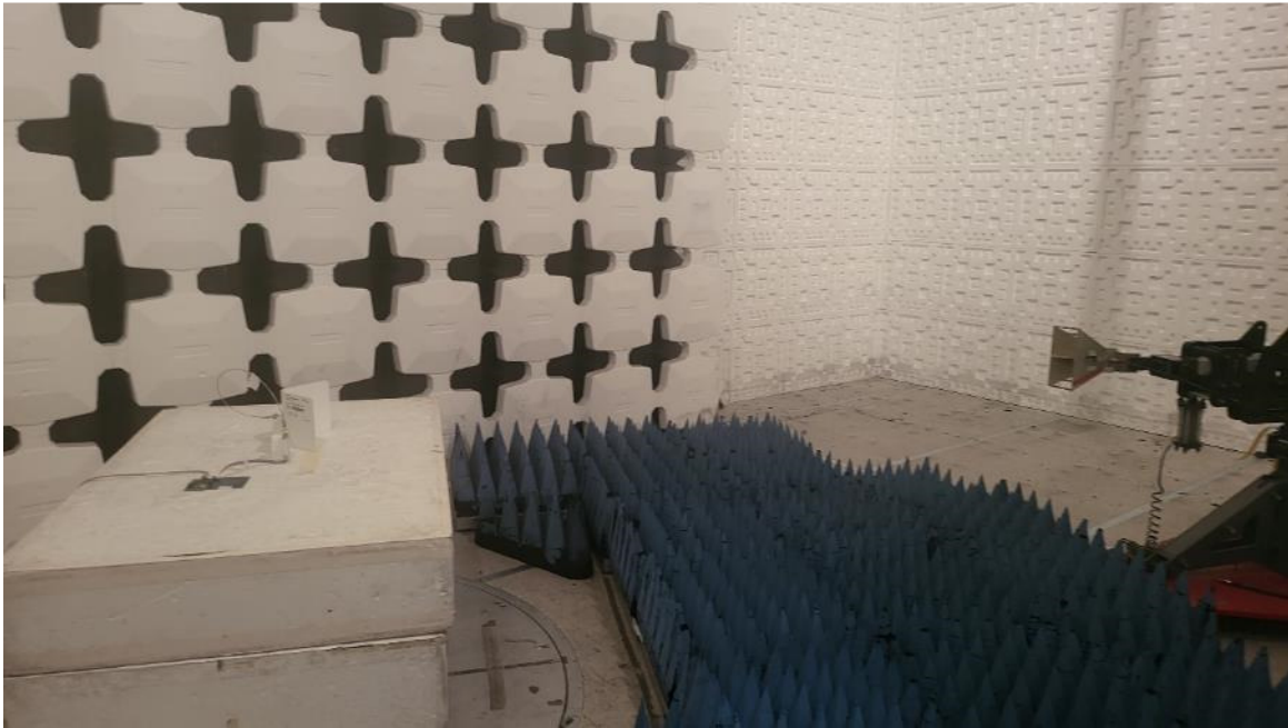
Figure 12. Radiated Emissions with Corner Reflector, above 1 GHz
