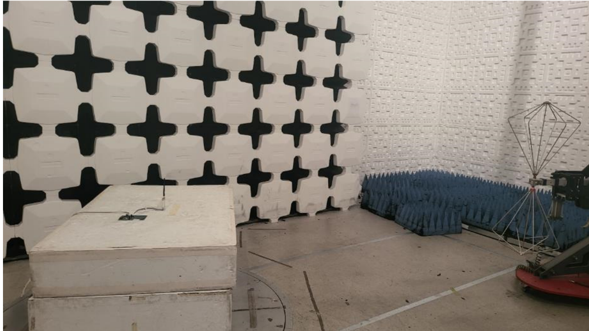
Figure 4. Radiated Emissions with Dipole, 30-1000 MHz
