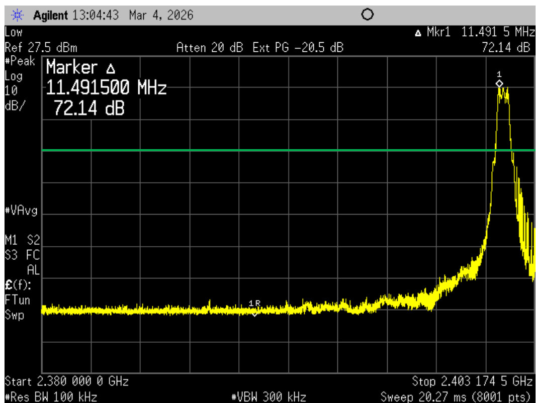
Figure 8. Authorized Band Conducted Band-Edge Compliance, Low Channel Delta, Hopping Turned OFF -Peak
