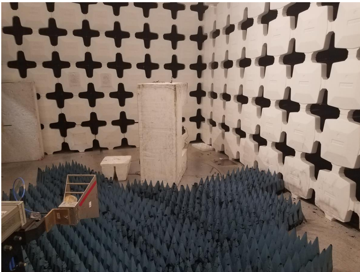
Figure 5. Radiated Emission Test Setup, above 1 GHz
