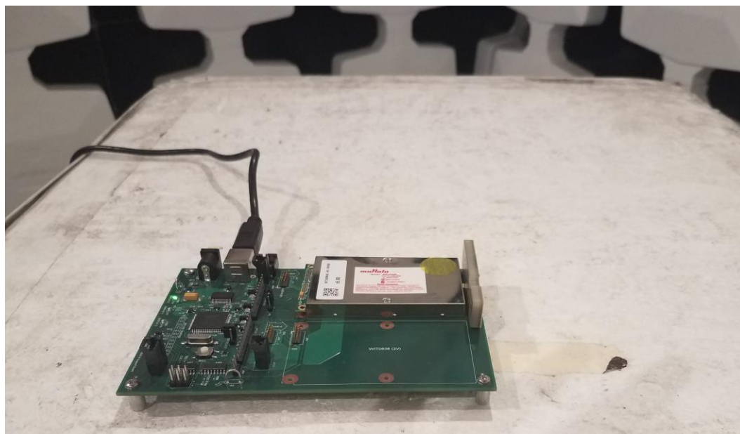
Figure 1. Radiated Emissions Test Setup, Patch Antenna
