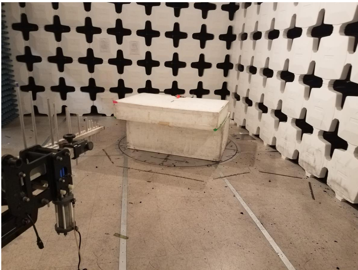
Figure 4. Radiated Emissions Test Setup, 200 MHz to 1GHz
