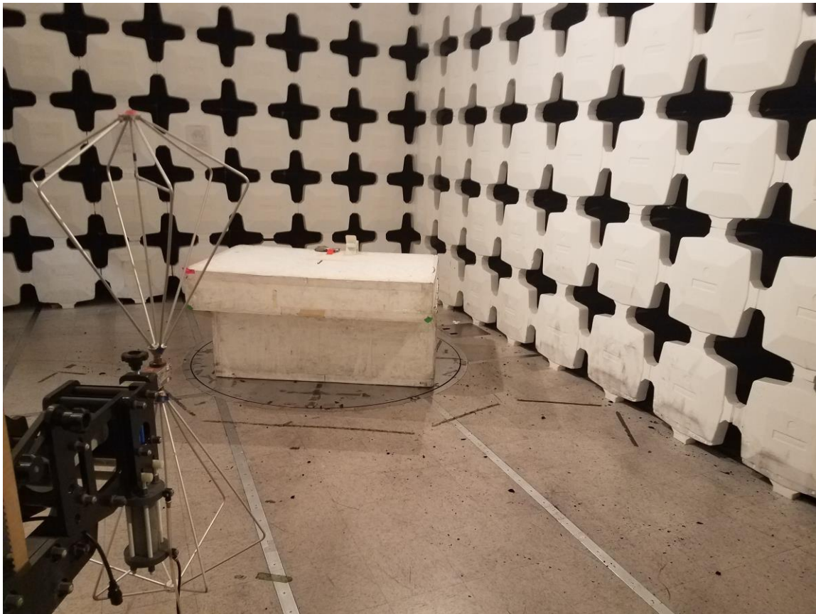
Figure 3. Radiated Emissions Test Setup, 30 MHz to 200 MHz
