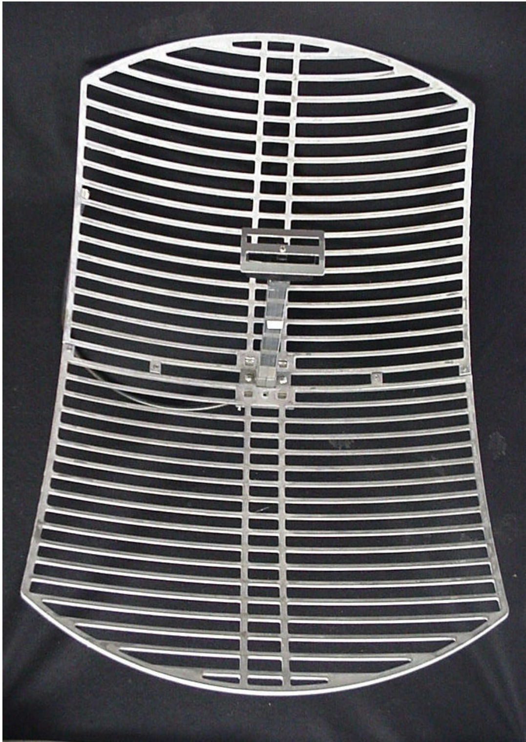
Photo 9. Parabolic Dish Antenna
