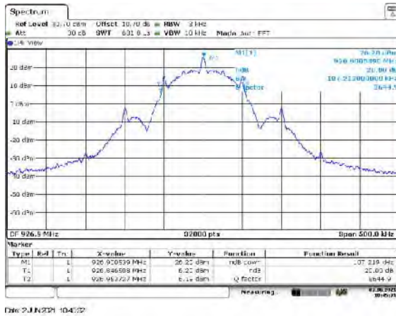
Figure 7.4.4.2-23: 20 dB BW High Channel – Mode 5
