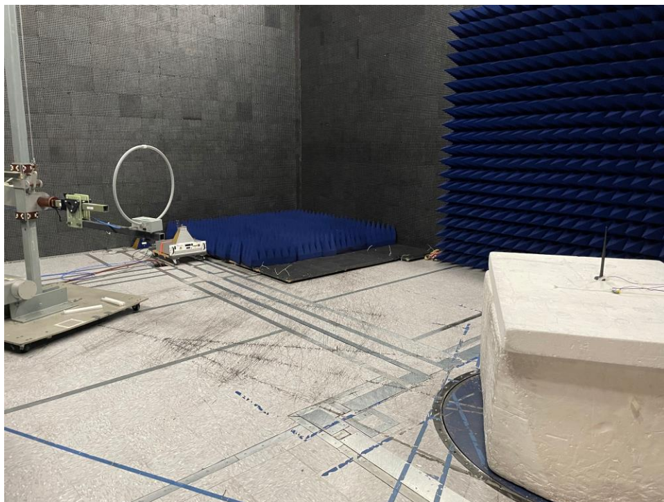
Figure 2: Equipment Under Test – Radiated Emissions <30MHz
