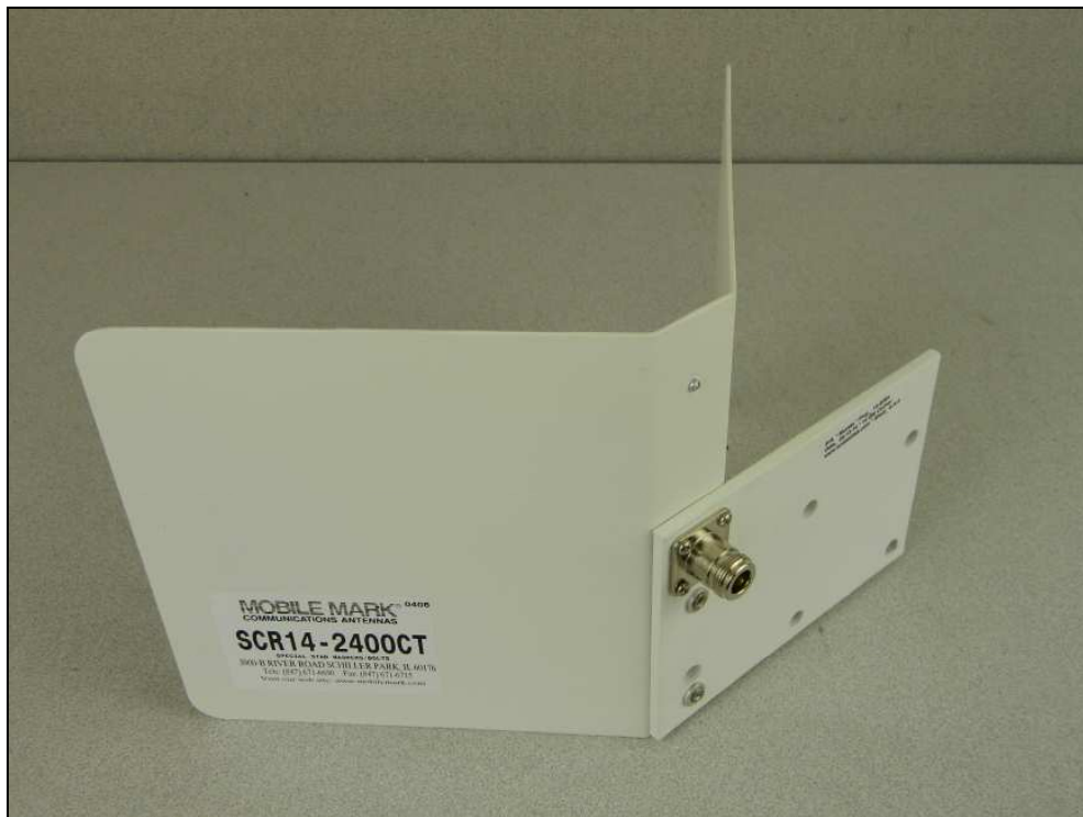
Figure 10: External Photo – Corner Antenna
