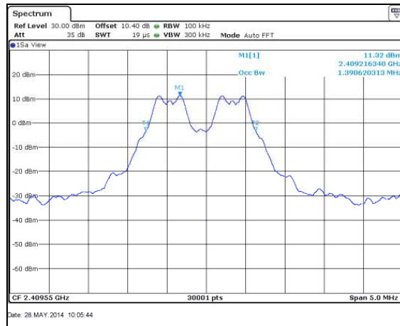
Figure 7.3.2-4: 99% Bandwidth Plot – LCH
