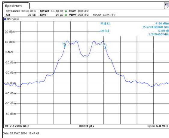
Figure 7.3.2-3: 6dB Bandwidth Plot – HCH
