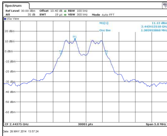
Figure 7.3.2-11: 99% Bandwidth Plot – MCH
