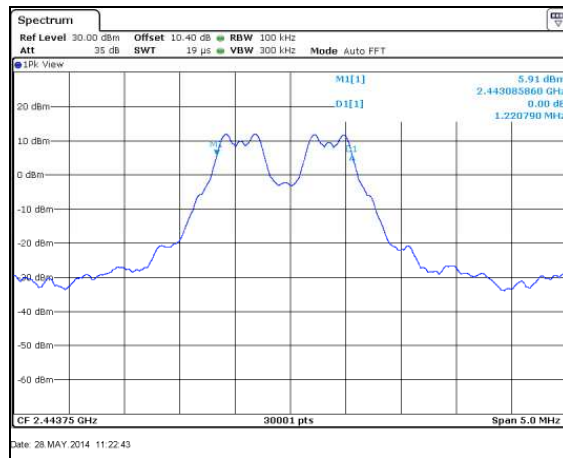
Figure 7.3.2-2: 6dB Bandwidth Plot – MCH
