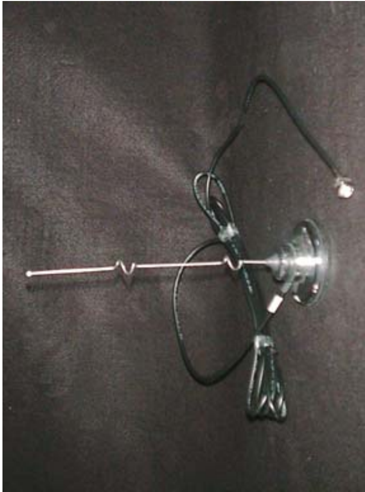
Photo 3. Antenna, MaxRad 5 dBi Whip (M/N MUF24005-RTNC)
