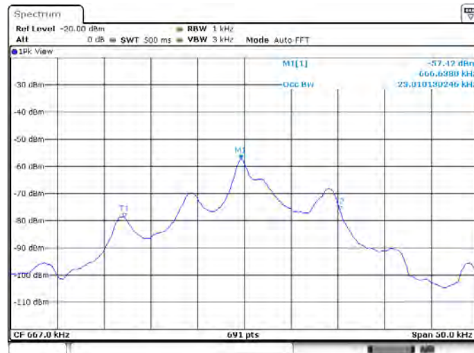
Emission Bandwidth Plot - 99% Bandwidth
