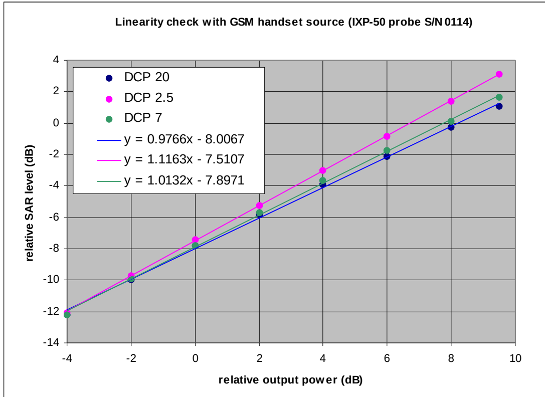
Figure 7. The GSM response of IXP-050 probe S/N 0114 at 1800MHz (max. SAR level 1.6 W/kg)
