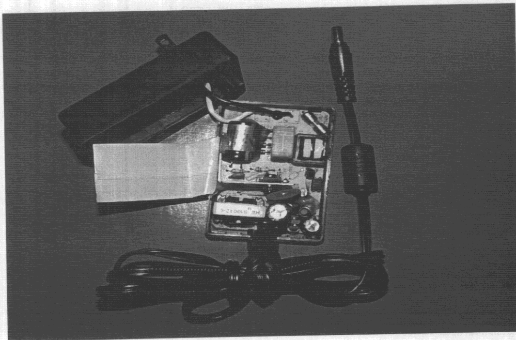
(14) INNER VIEW OF ADAPTOR (HiTRON)
