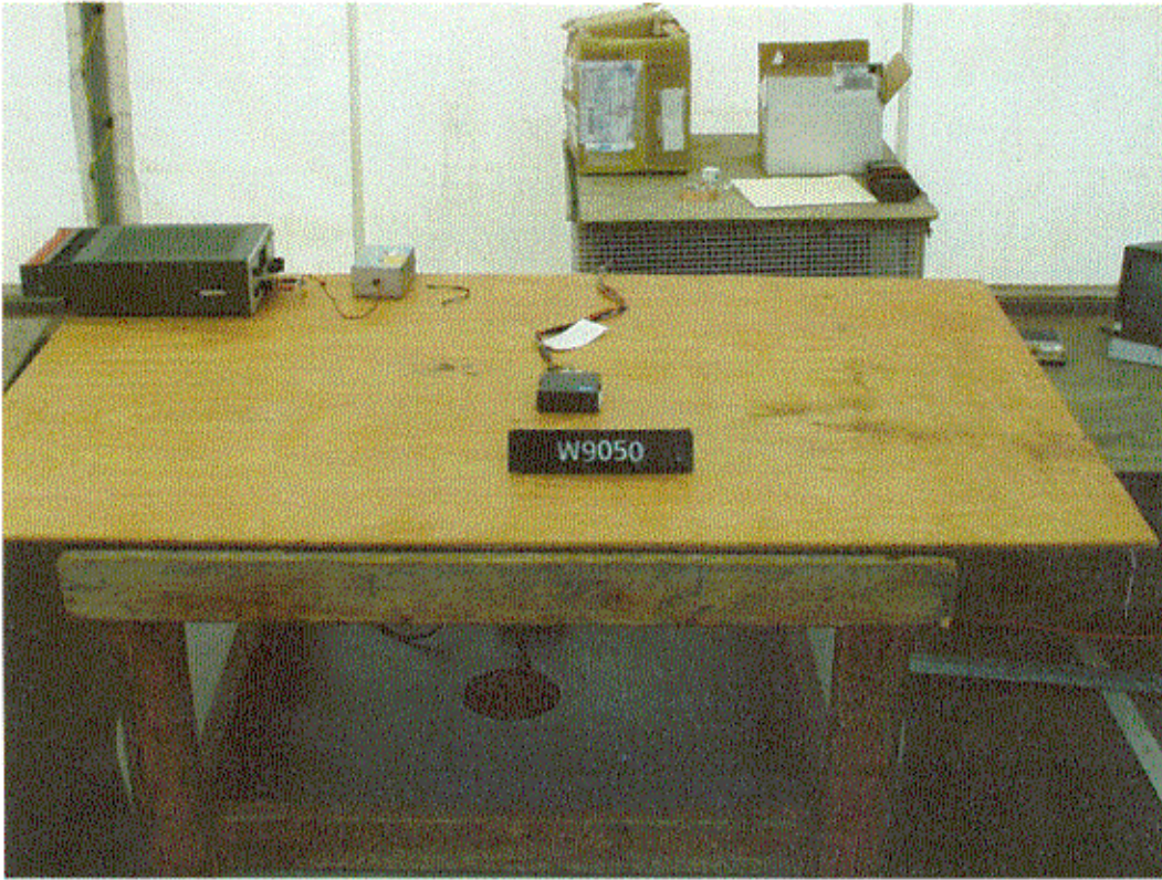
Test-setup photo(s): Radiated emission 30 MHz - 2000 MHz
