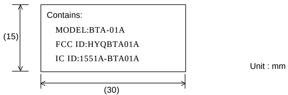
Fig. 4.6.2. FCC and IC ID Label layout
