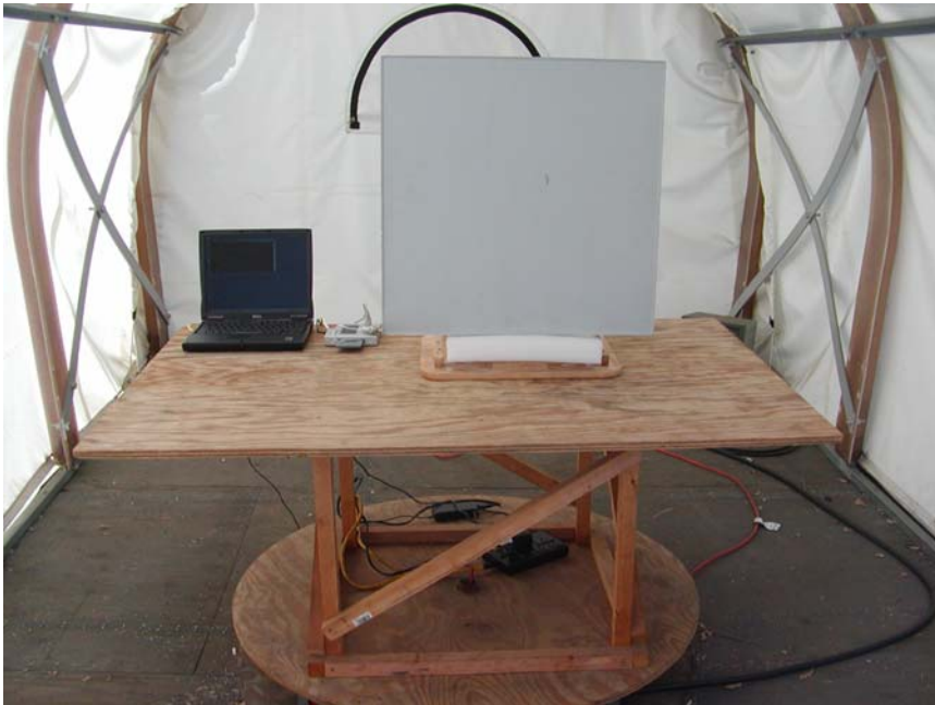
Radiated Emission with DFPD2-52 Antenna - Front View
