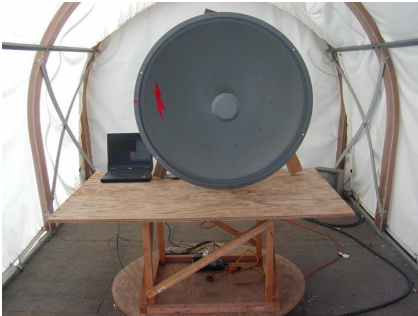
Radiated Emission with P3F-52-N7A Dish Antenna - Front View
