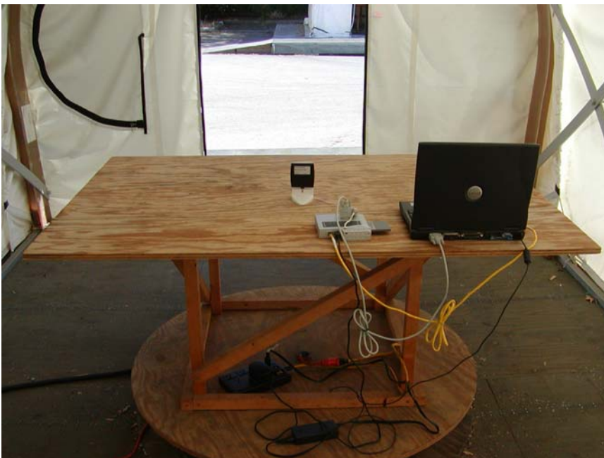
Radiated Emission with R0320-056 Antenna – Rear View
