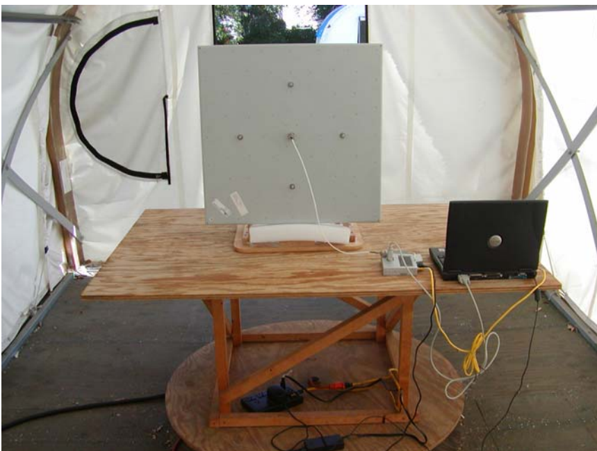
Radiated Emission with DFPD2-52 Antenna - Rear View
