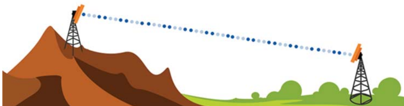
Figure 8-2 Typical installation showing device/antenna tilt angle
