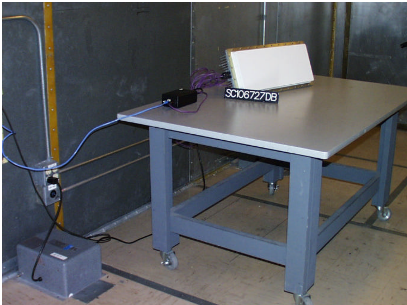
Photograph of Test Setup: AC Conducted Emission
