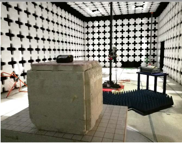
Radiated Emissions (>1GHz) – Rear View
