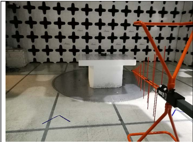
Radiated Emissions (<1GHz) – Front View
