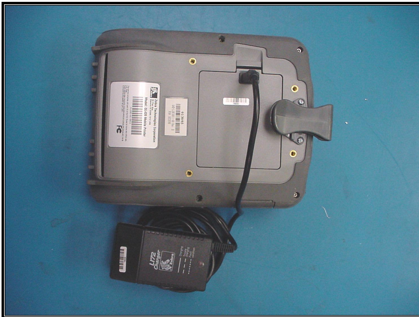
PHOTOGRAPH 2: BOTTOM OF EUT WITH FCC ID LABEL & WITH AC ADAPTER/CHARGER
