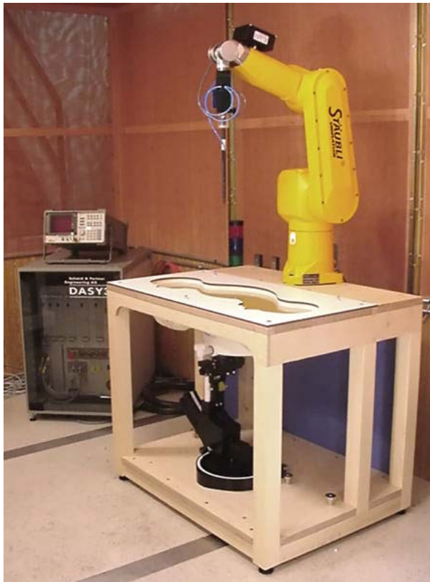
DASY3 SAR Measurement System with SAM phantom
