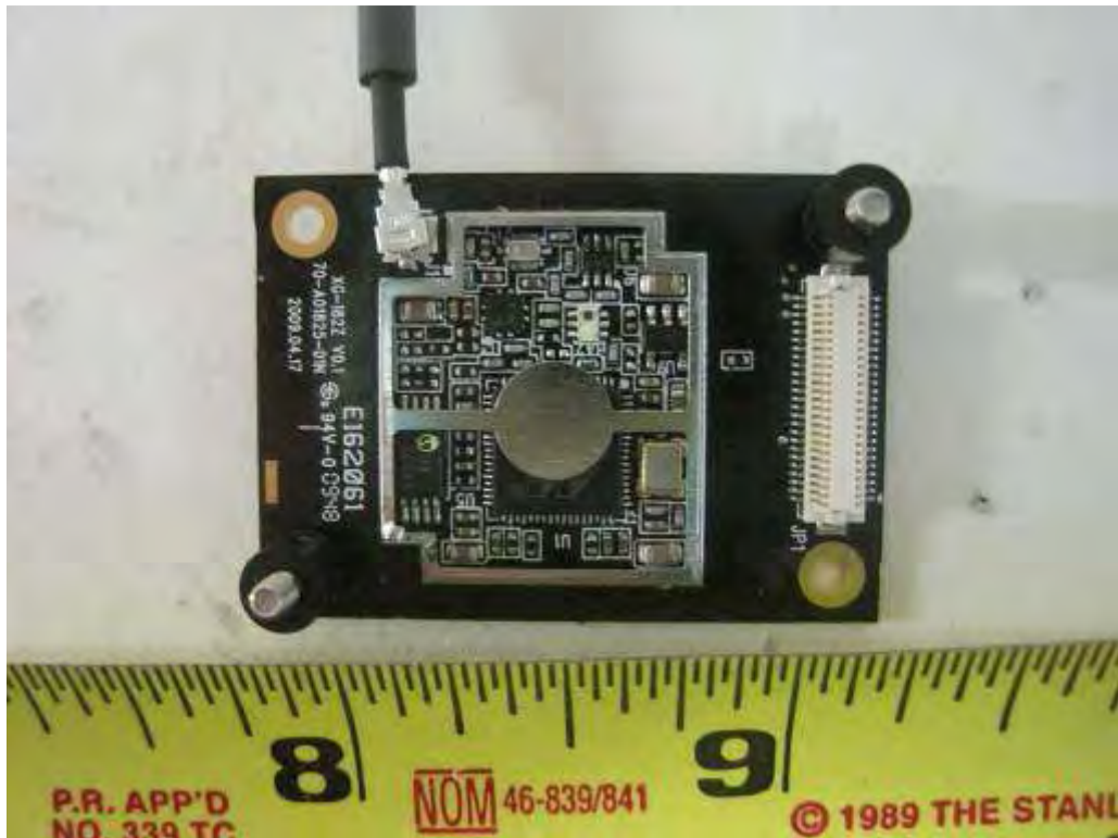
Radio Board shielding off View
