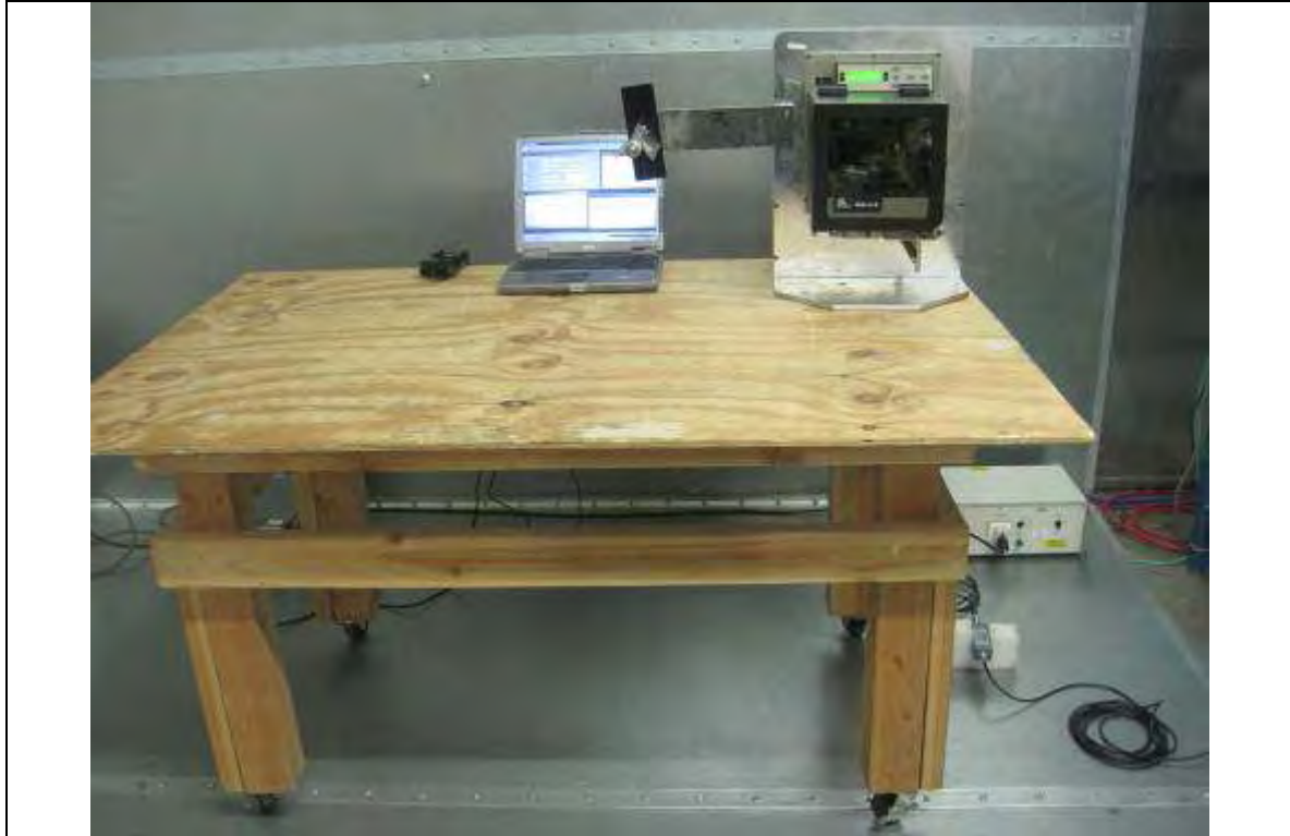
Conducted Emission Test Setup – Front View
