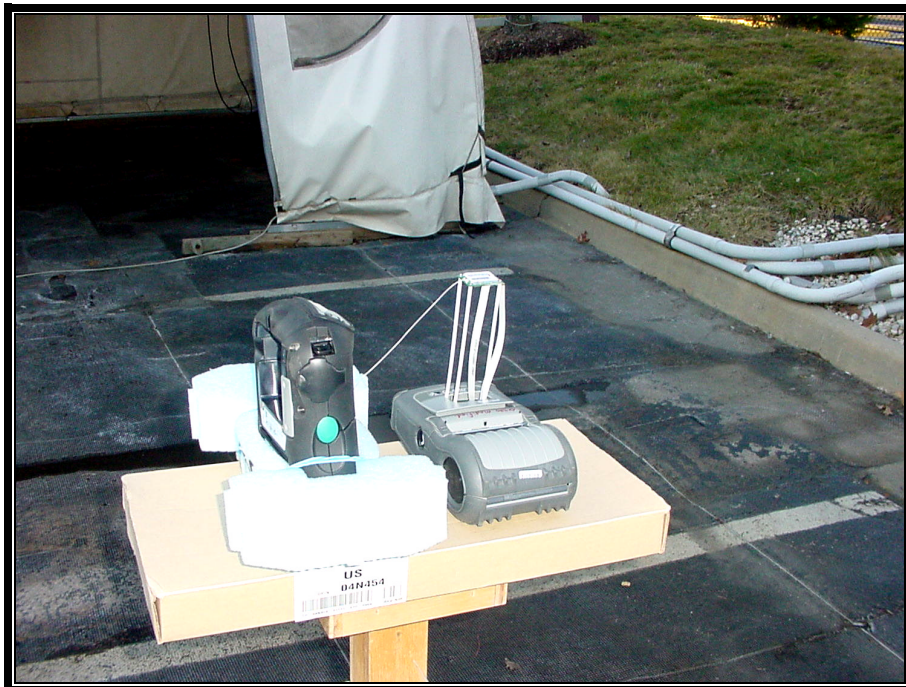
PHOTOGRAPH 8: RADIATED EMISSIONS REAR VIEW USING RW-420 CQ17252-1 ANTENNA
