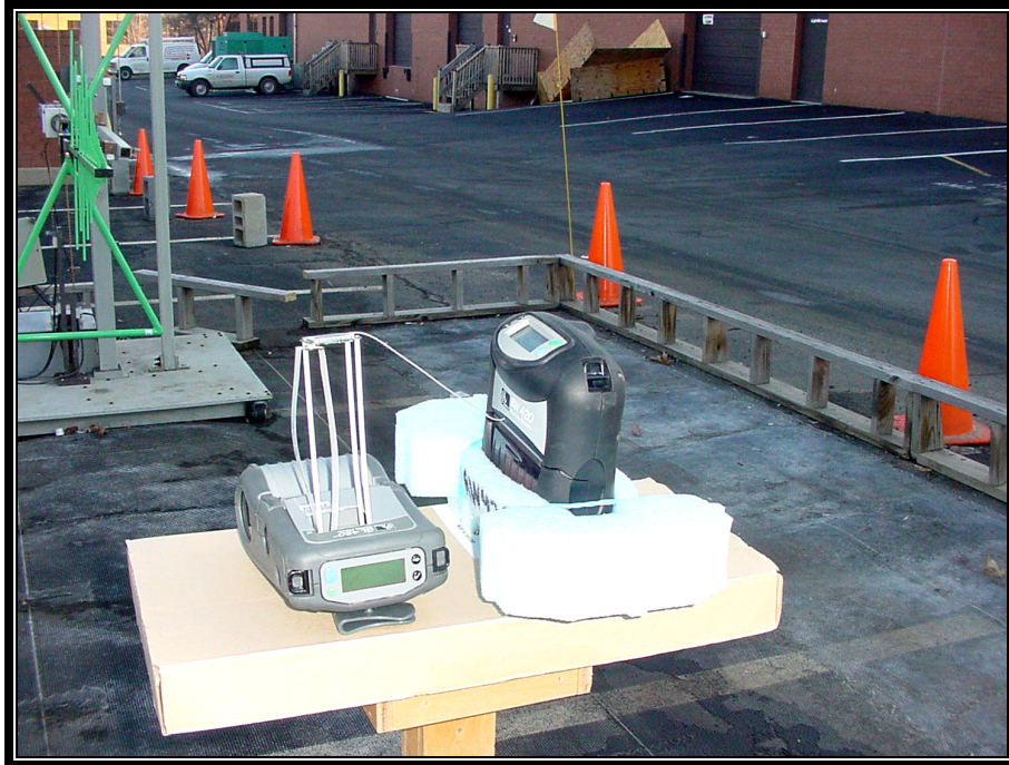
PHOTOGRAPH 7: RADIATED EMISSIONS FRONT VIEW USING RW-420 CQ17252-1 ANTENNA
