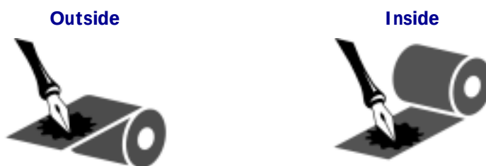
Figure 10 • Ribbon Coated on Outside or Inside
