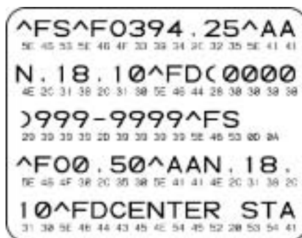
Figure 54 • Communications Diagnostics Test Label
