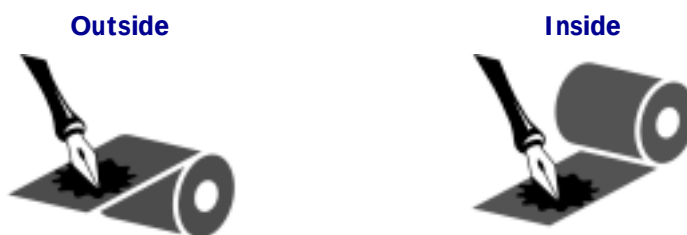
Figure 10 • Ribbon Coated on Outside or Inside
