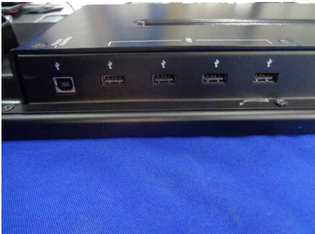
Figure 6 I/O Port of the EUT
