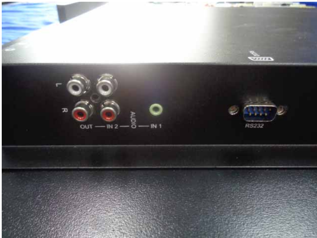
Figure 7 I/O Port of the EUT
