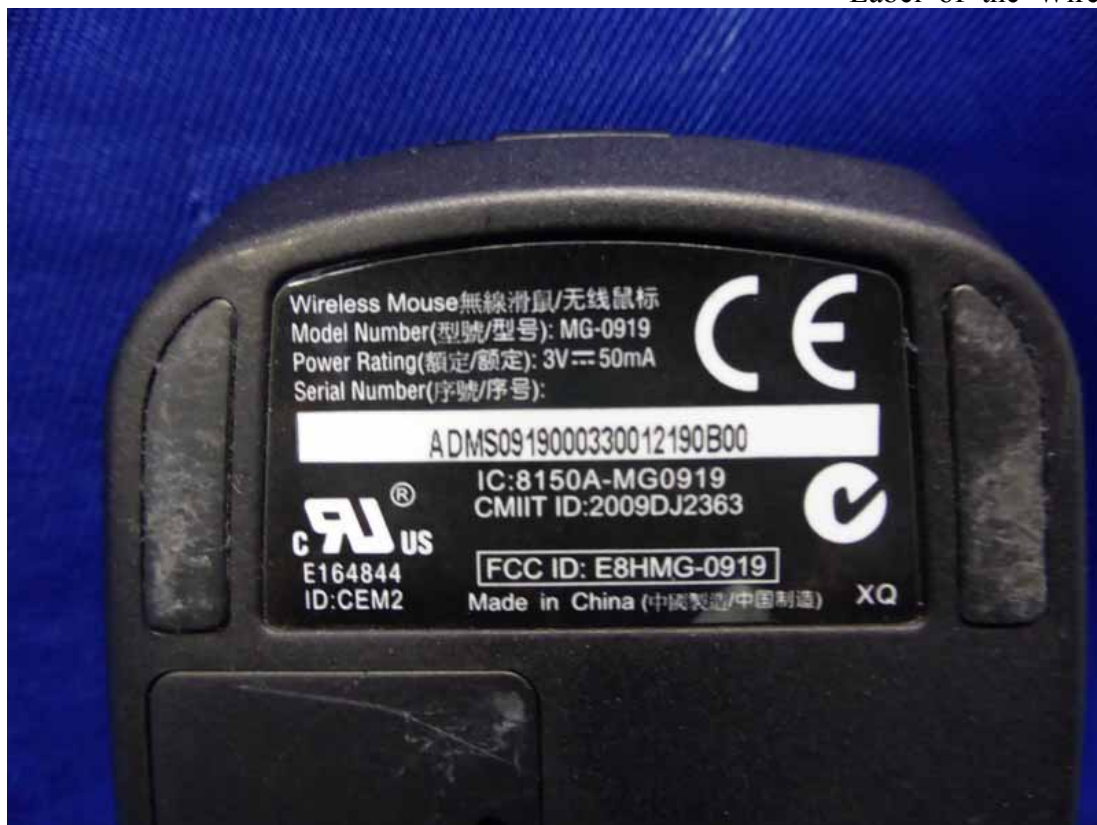
Figure 31 Label of the Wireless Mouse
