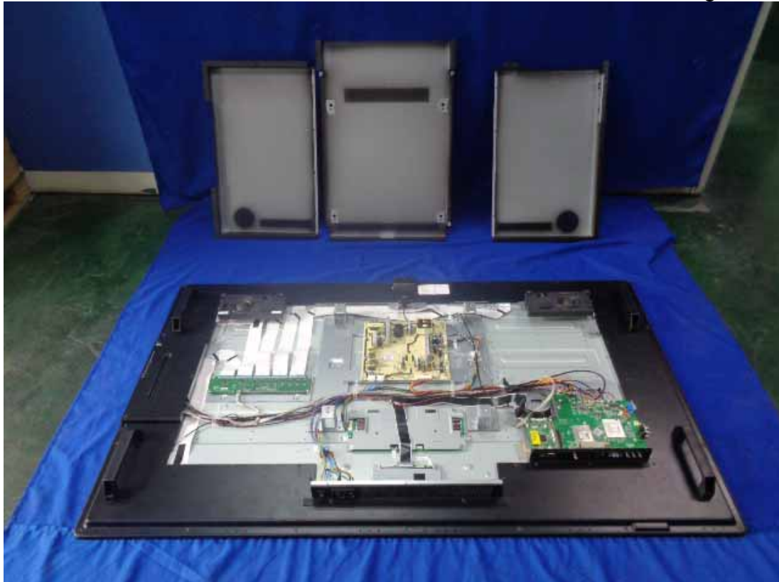
Figure 9 Inside Configuration of the EUT
