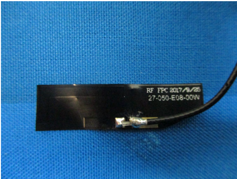
FPC Antenna – View
